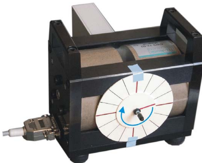
Figure 31. Home-made goniometer for gypsum monocrystal study attached to the electromagnet.
